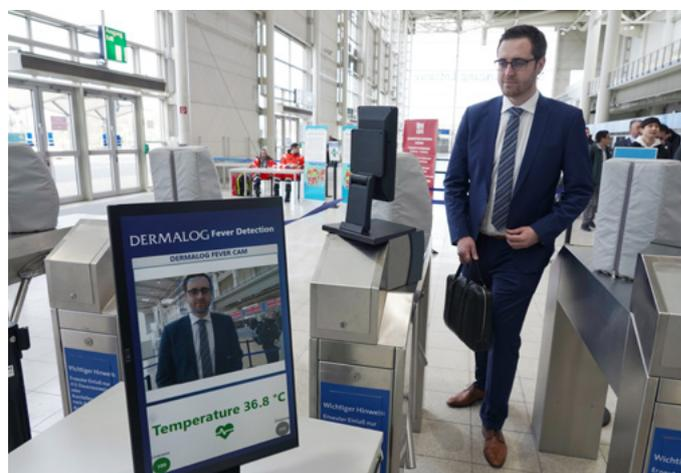
The DERMALOG system detects in real time the temperature of each visitor as he passes through the entrance and sends the measured values to the control staff via screen notification.
